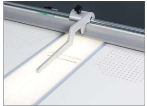
Scaled light table, positioning line, suction assistance and interchangeable spine guides
