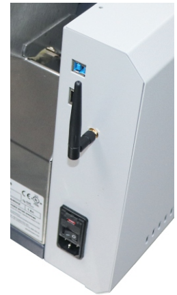
Three PC interface ports: USB 3.1, Ethernet, WiFi
