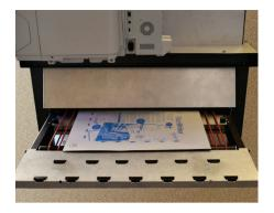
The imaged plates are manually fed through the integrated finishing unit which dries the plates and bonds the liquid dots to the plate surface.
