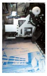
The imaged plates are manually fed through an integrated finishing unit to dry the plates and bond the liquid dots to the plate surface.
